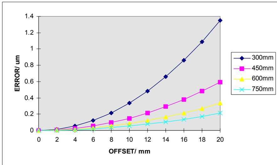
Figure A1.4. Error between measured and true camber of 150 micron, due to offset from true diameter.
