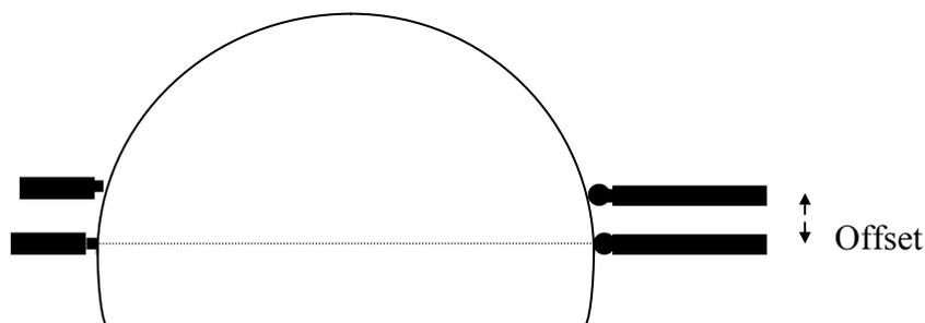
Figure A1.3. Error due to offset of LVDT and follower.
