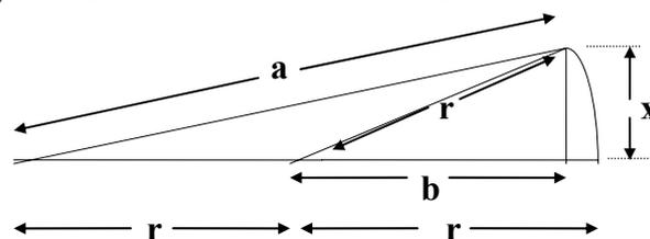
Where  $r$  = radius,  $x$  = offset and  $\text{error} = 2r - a$ . For example, for a roll of diameter 450mm and offset 5mm, the error is calculated as;
