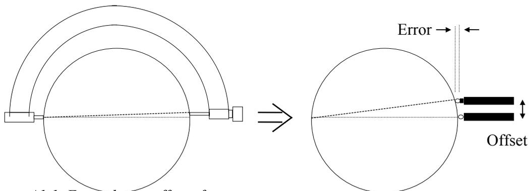
Figure A1.1. Error due to offset of a micrometer.
