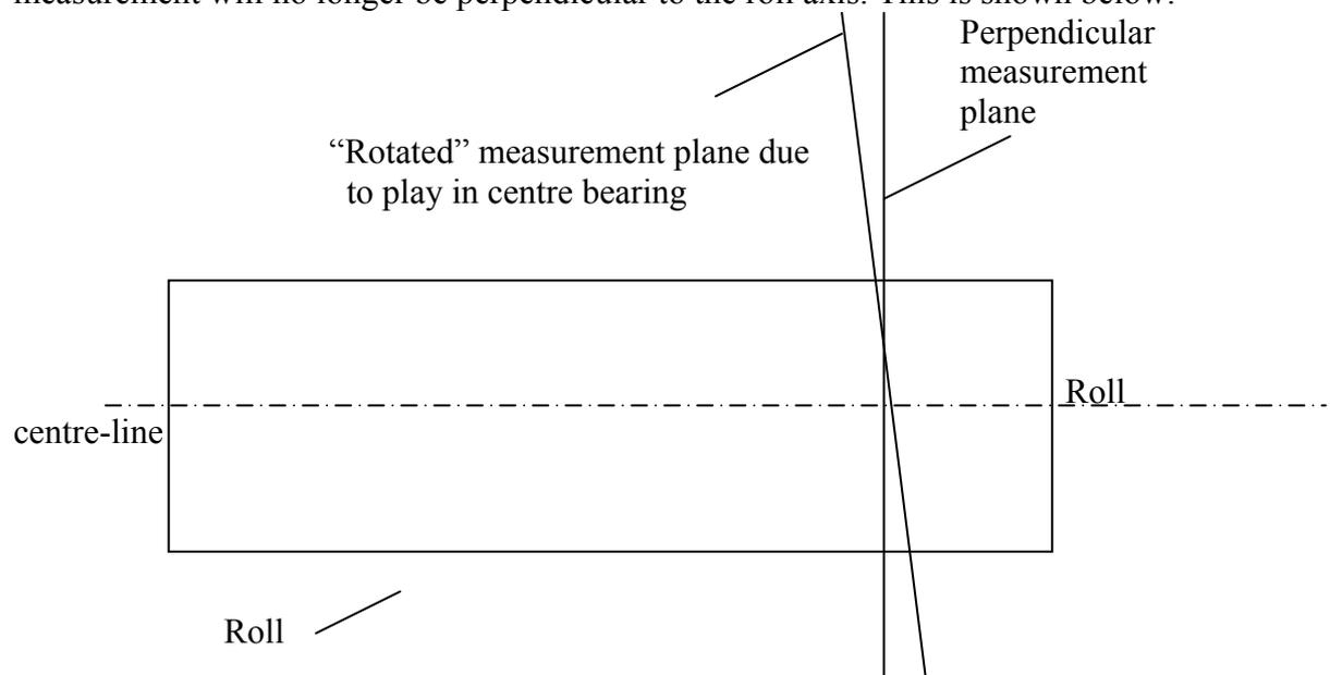
This will cause a slight depression of the LVDT probe tip, and so introduce an error to the measurement. For this reason, the centre bearing is adjustable and *it is essential that this is checked and adjusted at quarterly intervals when the calibration takes place.*
