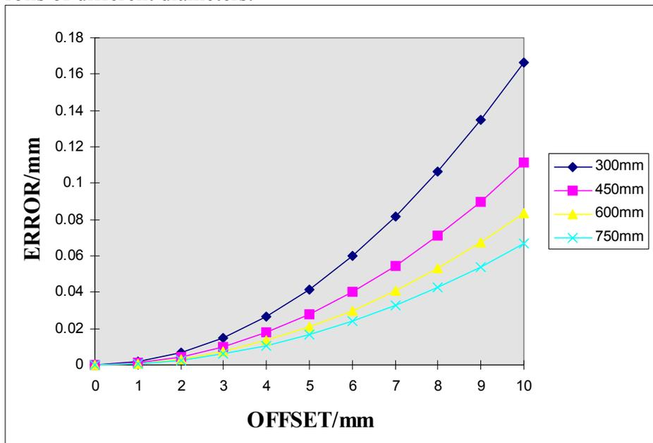
Figure A1.2. Error due to offset for various diameter rolls.
